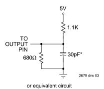
Figure 1. Output Load
