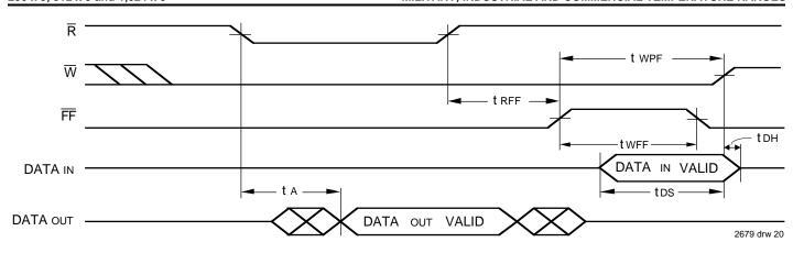
Figure 18. Write Data Flow-Through Mode
