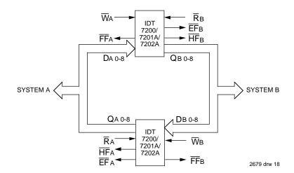
Figure 16. Bidirectional FIFO Mode
