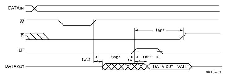
Figure 17. Read Data Flow-Through Mode
