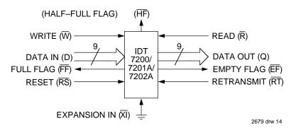
Figure 12. Block Diagram of Single 256 x 9, 512 x 9, 1,024 x 9 FIFO
