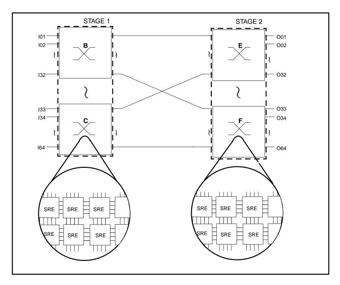
Fig. 2 - Example of a large switch configuration
