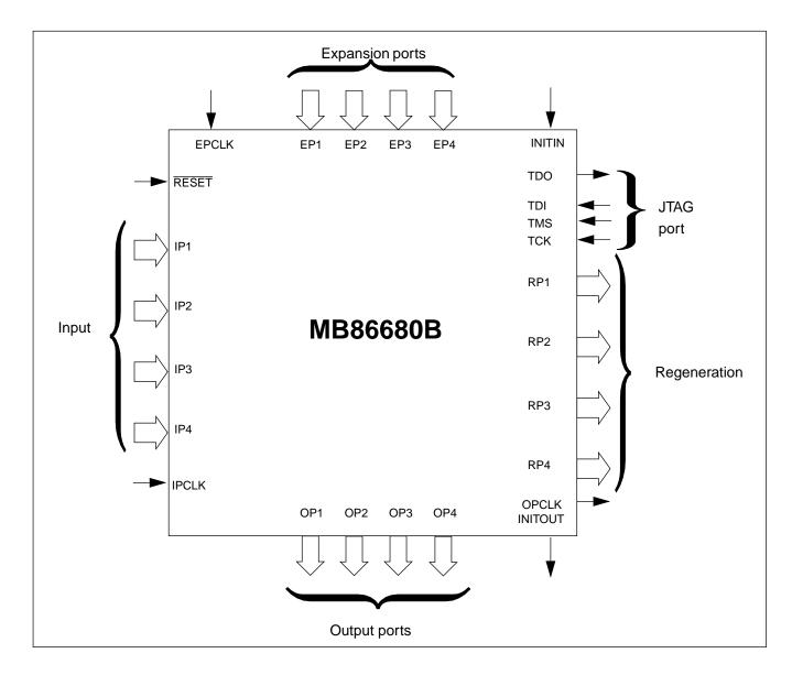
Fig. 3 - MB86680B I/O Block Diagram
